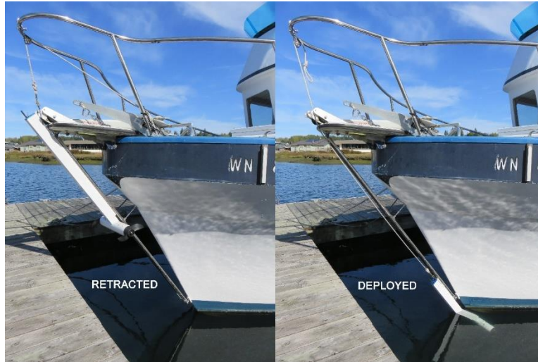
Figure 5: Thruster Retracted (Motors inhibited) and Deployed (Motors armed and ready)
